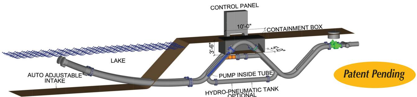
Remote or Auto Adjustable Intake on Long Reach Intake to In-Ground Wet Well, No Building Required
