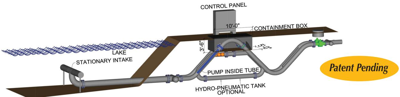
Stationary High Volume 22,000 GPM Single Intake to In-Ground Wet Well, No Building Required
